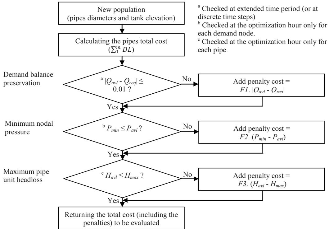
Fig. 2. Objective function in EO algorithm (NetOpt model)
