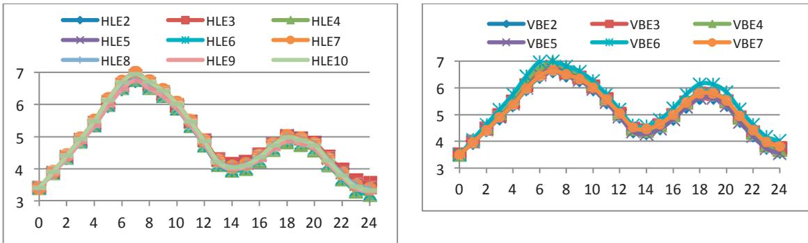
Fig 7. Tank volume variation: Y-tank depth (m), X - time (hours)
